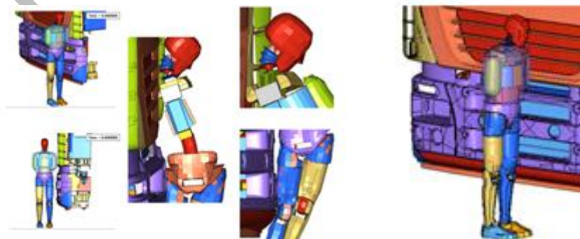
Figure 22. PAC dummy: numerical simulations of pedestrian-to-truck collisions done within APROSYS project
