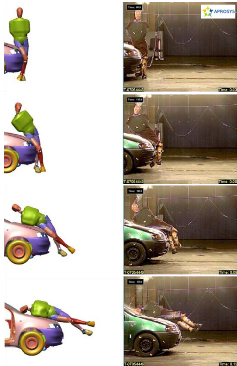
Figure 21. PAC dummy: experimental and numerical model comparison done within APROSYS project
